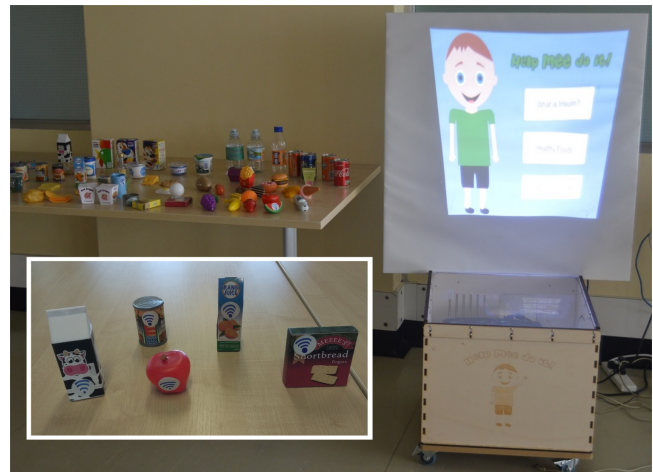
Figure 5: The educational tool comprises of a projection that interacts through RFID sensors with the plastic food toys and the toy insulin pen.
