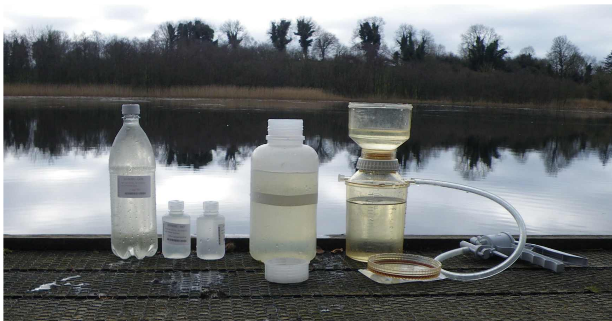
Figure 5 Water sample collection and Nalgene filtration unit (right)
