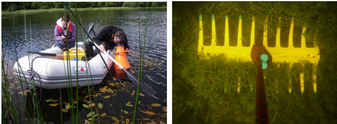
Figure 2 Sampling methods: bathyscope (a) and double-headed rake (b)
