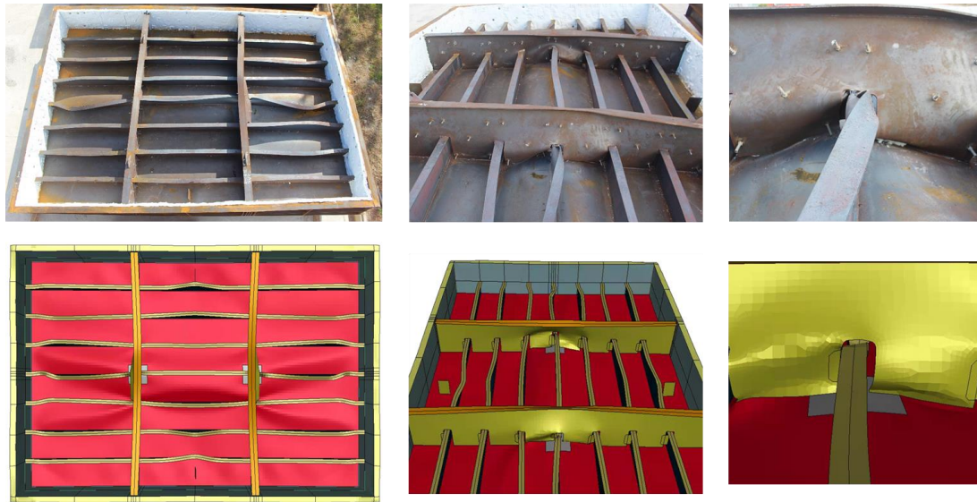
Figure 19. Comparison of the deformed shape for the structure with PFP after the collapse between the tested structure and the computation.
