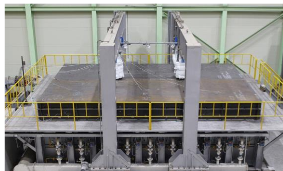
(b) Stiffened plate structure on the furnace
