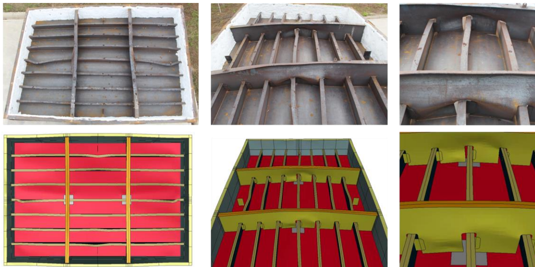
Figure 18. Comparison of the deformed shape for the structure without PFP after the collapse between the tested structure and the computation.
