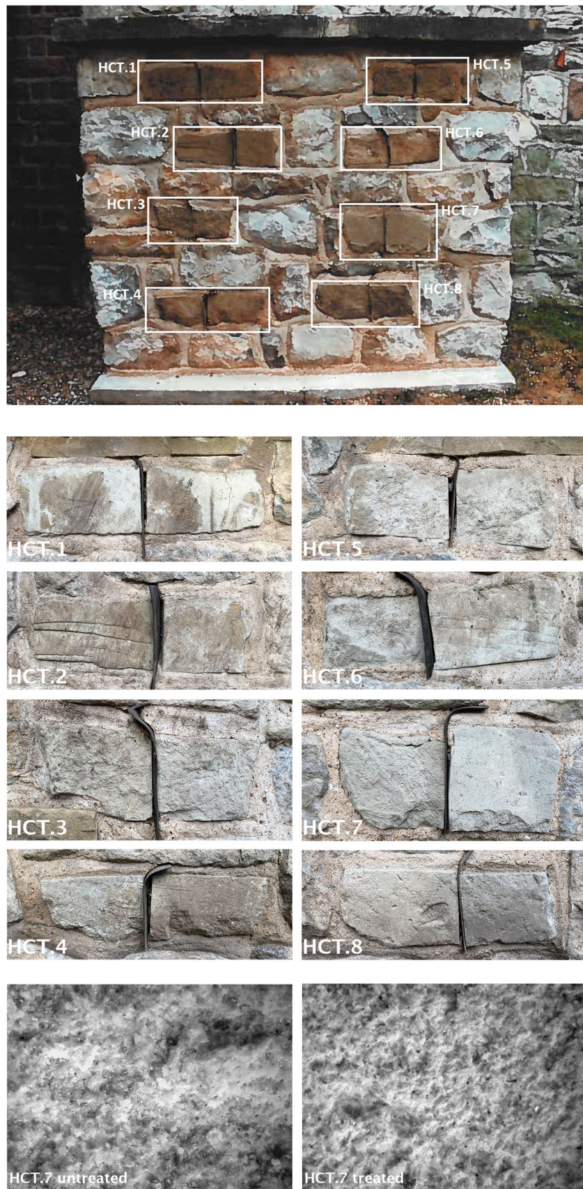
Figure 4. HCT trial wall at ToL. Top: shortly after treatment in 2001 (dark surfaces due to residual moisture following treatment). Middle: individual stones in 2018 (each stone treated on right hand side only). Bottom: micrograph taken with Dinolite USB microscope, showing consolidation of treated surface.
