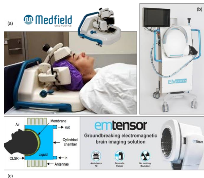
Figure 1-19: Novel MWI Devices. a) The StrokeFinder MD100 (from medfielddiagnostics.com). b) The EMvision (from EMvision.com). c) The EMTensor (from EMTensor.com).
