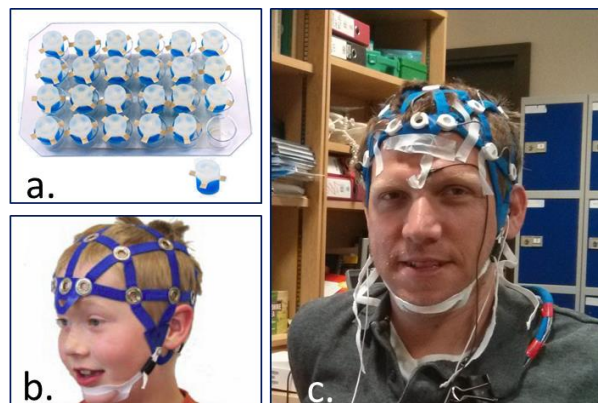
Figure 2-8: Hydro-Gel Electrodes. a) Hydro-gel bio-sensors ( http://hydrodot.wix.com ) b) Typical set-up ( http://hydrodot.wix.com ) c) Set-up in this study.
