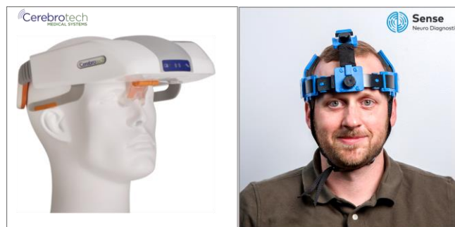
Figure 1-20: Novel RF-based Devices. Left: The Visor device (from cerebrotechmedical.com ), Right: The Sense device (from senseneuro.com ).
