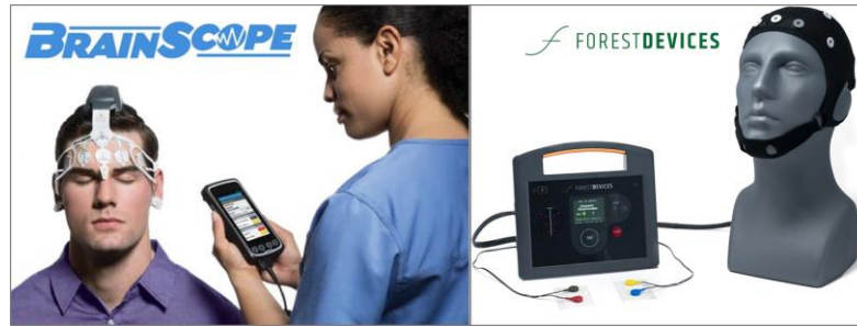
Figure 1-17: Novel EEG Setups for Stroke Diagnosis. Left: the BrainScope (from brain-scope.com), Right: the AlphaStroke (from forestdevices.com)
