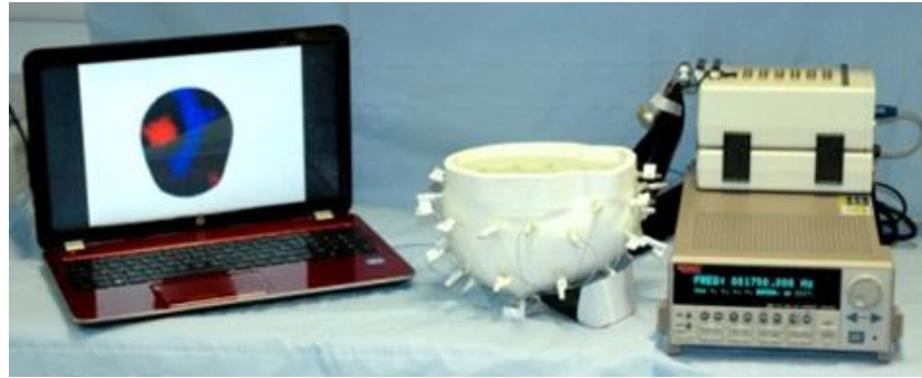
Figure 1-4: The UCL ScouseTom EIT System in Tank Experiment
