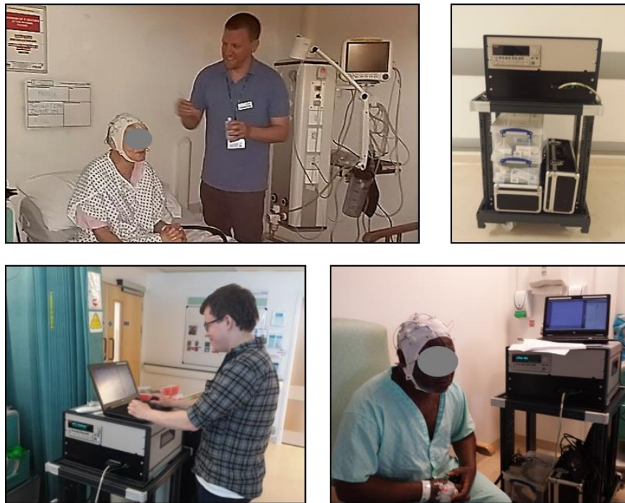
Figure 4-9: Images of the Clinical Set-up at UCLH HASU. Top left – applying electrodes to a bed-sitting patient. Top right – The UCL ScouseTom 2.5 EIT system in its hospital version, fully stacked for bedside data collection. Bottom-left – Running the ScouseTom near a patients’ bed. Bottom right – full running set-up on a chair-sitting patient at UCLH HASU.
