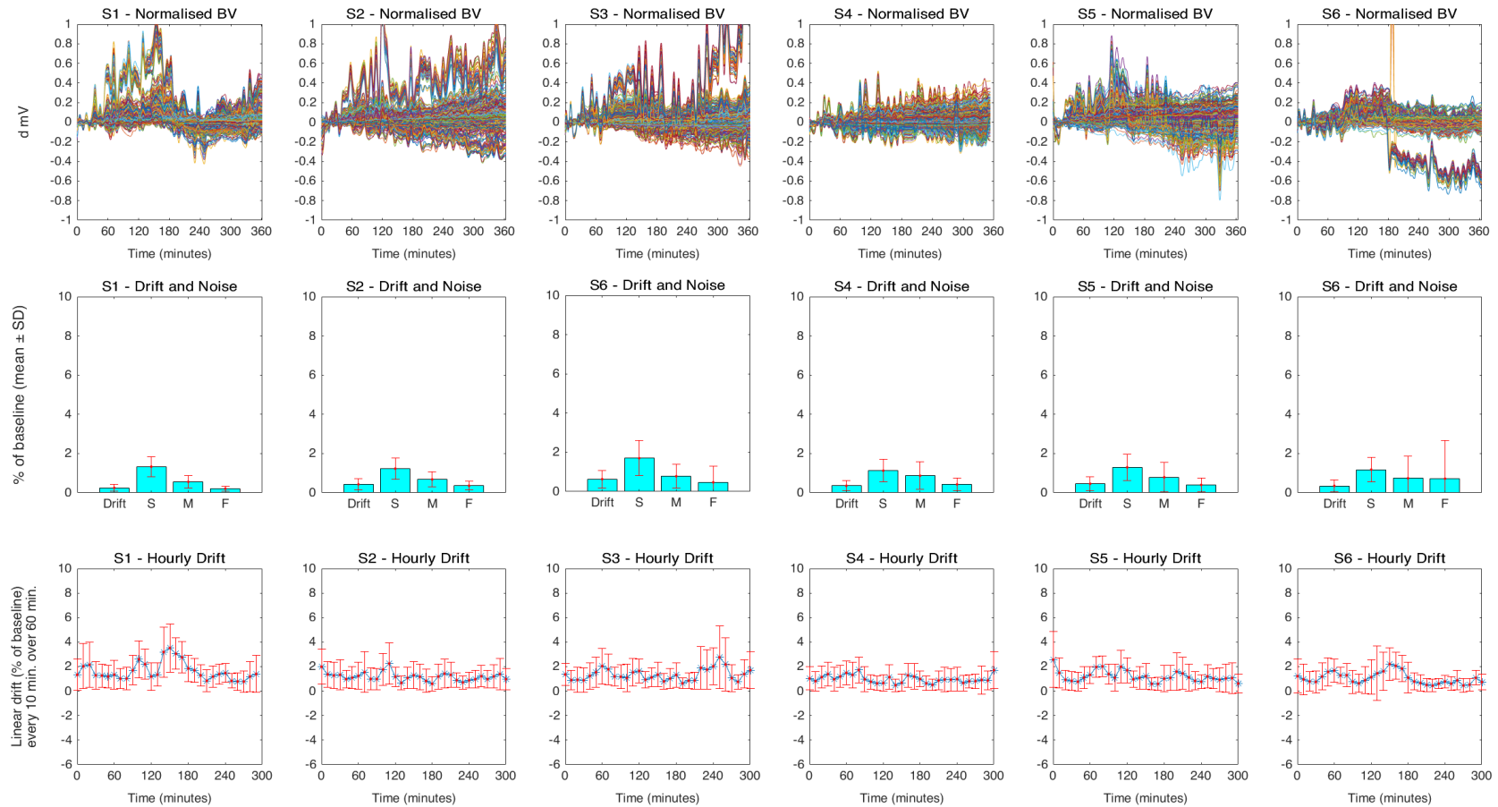
Figure 2-18: Common Reference Measurements (Best 90% Combinations). Each column represents one of the six subjects. The upper row presents the change in recorded raw BV over time in milliVolts. The middle row summarises the average hourly drift and the noise (slow changes, middle band changes and high frequency noise) over the complete length of the recording, in percentage from baseline BV. Red error bars are \pm 1SD . The lower row describes hourly drift - change in linear drift over time, by calculating drift over the next 60 minutes. This is done repeatedly every 10 min. Blue asterisks represent the mean across combinations, red errors bars \pm 1SD .
