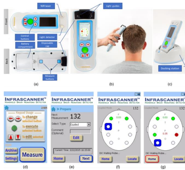
Figure 1-18: Novel NIRS Device. a) Infrascanner 2000 handheld battery-operated sensor, front and back. b) Disposable cap with light guides for NIR laser and detector positioned over scalp. c) An optional docking station for data backup and/or battery recharge. d) Home screen. e) Preparation screen at the beginning of a session. f) Typical measurements completed at frontal lobe at two locations. g) Measurements completed at parietal lobe with simulated head trauma. [18]
