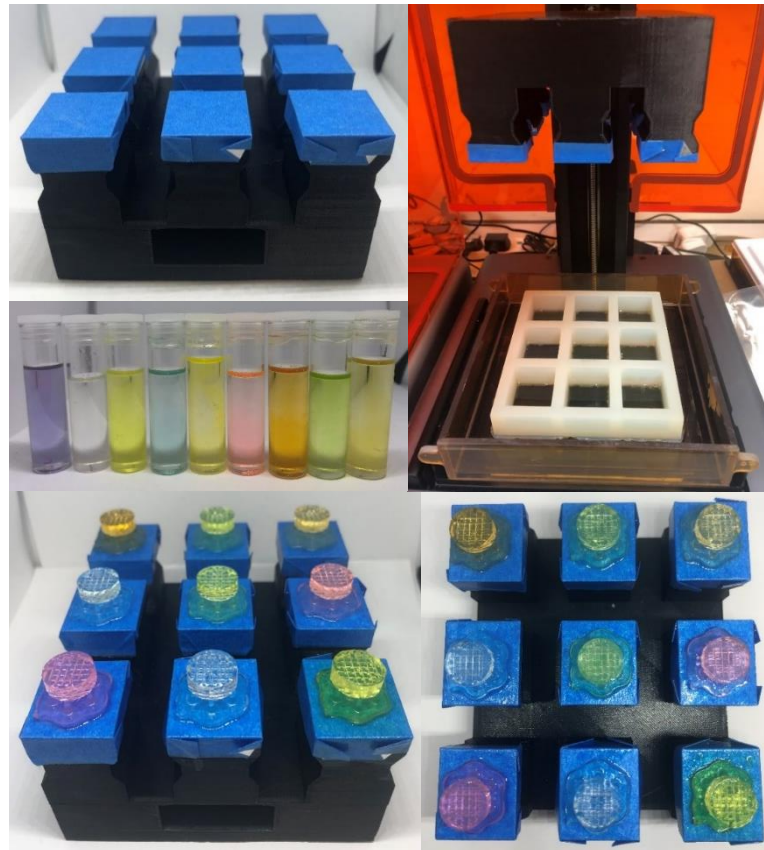
Figure 78 – Images showing an adapted Formlabs Form 1+ SLA 3D printer setup including 9 printheads and printing wells, and successful multi-material printing of 9 small objects
