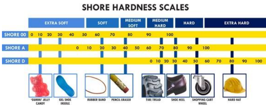
Figure 42 – Shore hardness scales. Reproduced from Albright Silicone webpage (2015) 228 .
