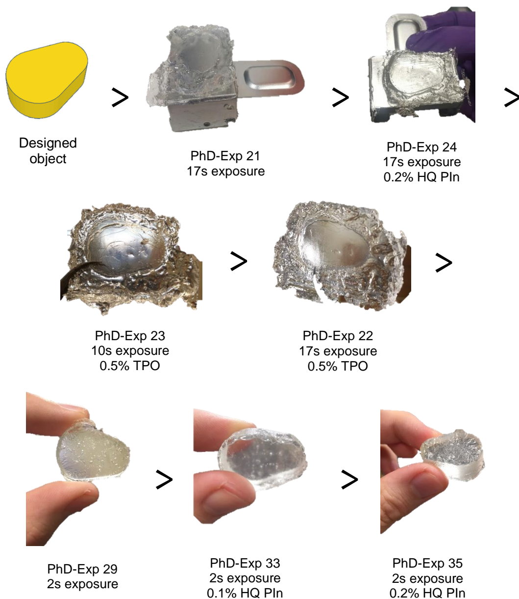
Figure 81 – Images showing multiple consecutive prints utilising a PEG575DA + trithiol + 1% TPO (unless stated otherwise) formulation with varying layer exposures and amounts of photoinhibitor HQ.
