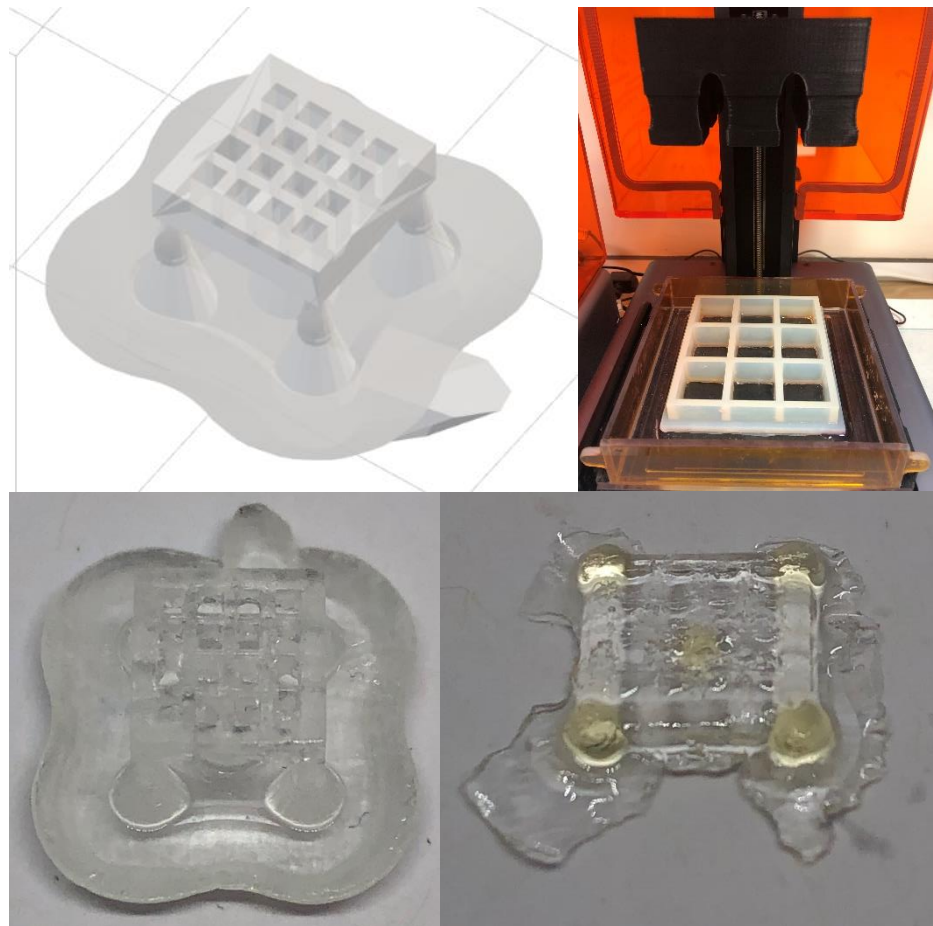
Figure 79 – Top left image shows desired object for printing in Formlabs PreForm software. Top right image shows print setup using an adapted print head and print tray. Bottom left image shows successful print using Formlabs Clear V4 resin. Bottom right image shows failed printing using a TEGDVE + 3% P3C-P formulation.
