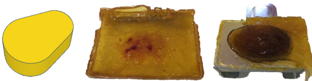
Figure 80 – Left image shows desired object, generated using Tinkercad, for printing. Middle and right images show subsequent failed prints using a TEGDVE + 5% w/w P3C-P + 3% benzoyl peroxide formulation on the MiiCraft+ SLA 3D printer
