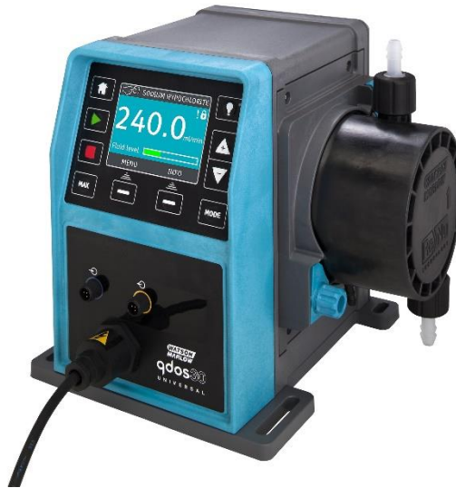
Figure 2.4: High accuracy water pump, model qdos03 supplied by Watson Marlow, that was used to provide water in the shower spec cleaning apparatus. It is a versatile peristaltic chemical metering pump, which is able to provide a range of flowrates from 0.1 – 500ml/min at a steady pressure of 100psi.
