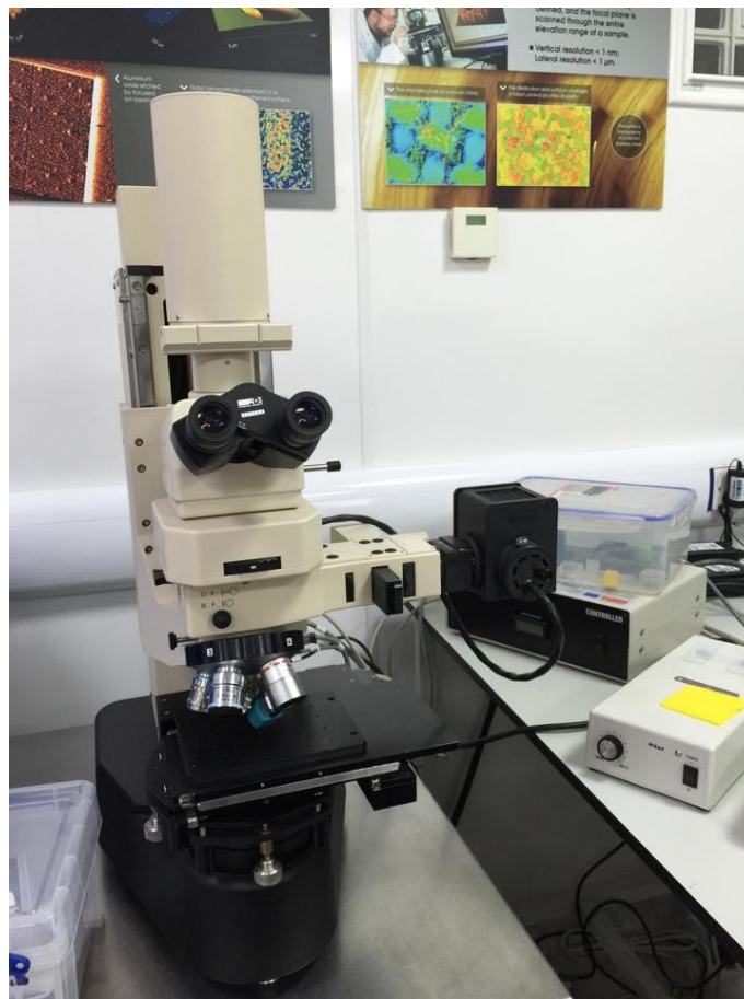
Figure 2.7: Interferometer set up, showing the main microscope, the light source controller and the intensity control.
