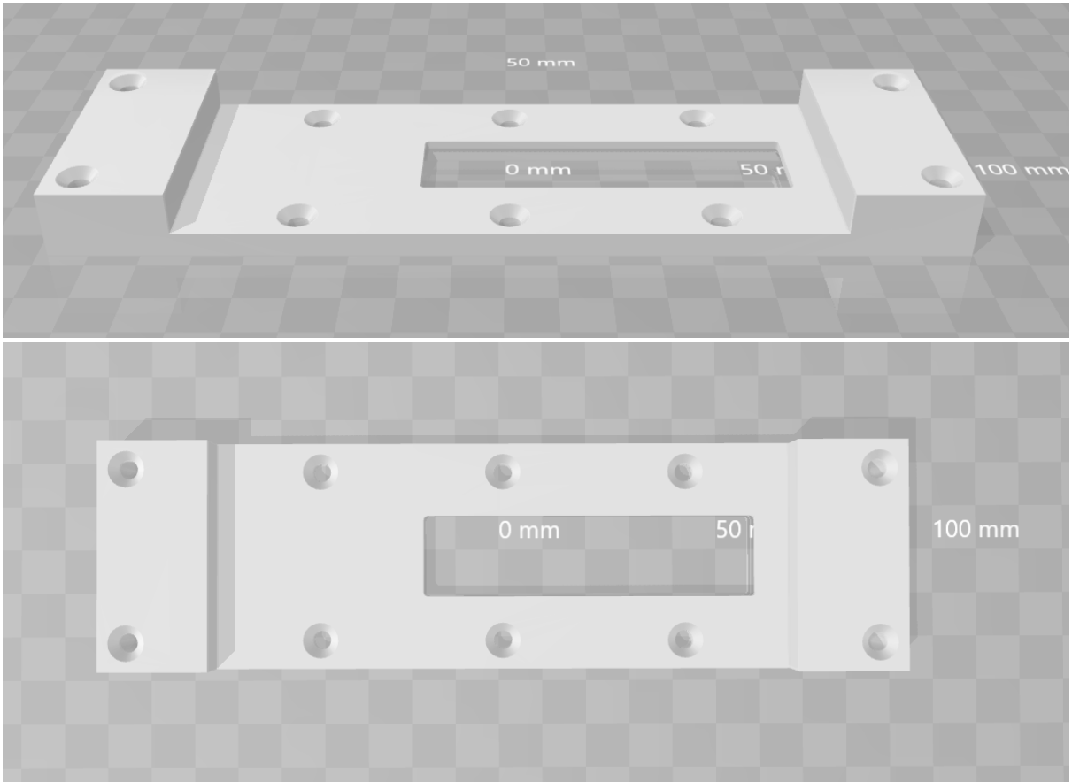
Figure A.2: Water flow chamber upper part. In this design, there is a hole where a glass is supposed to be glued so that the rinsing of the substrate can be monitored. The two boxes at both ends of the chamber are hollow and work as water tanks to eliminate turbidity coming from the water input cable and allow laminar flow in the chamber.
