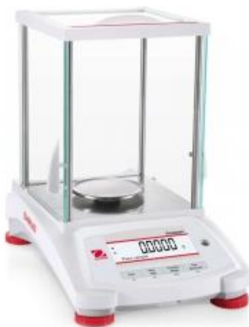
Figure 2.1: Ohaus analytical balance that was used for gravimetric analysis of this project.
