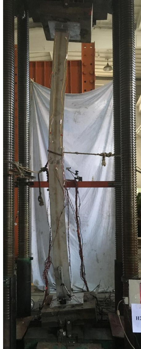
(b) H 304-2500 specimen failing about the minor axis
