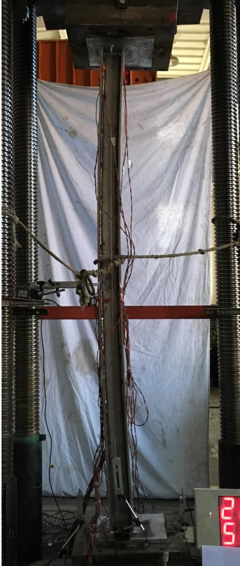
(a) I 304-2500 specimen failing about the major axis
