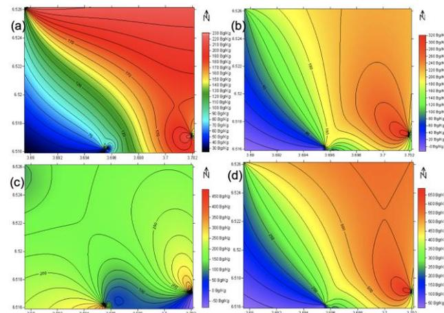
Figure 5: Radiological Map of the Study Area Showing; A)  $^{238}\text{U}$  Activity Concentration (Bq/Kg); B)  $^{232}\text{Th}$  Activity Concentration (Bq/Kg); C)  $^{40}\text{K}$  Activity Concentration (Bq/Kg); and D) Absorbed Gamma Dose Rate (Ngyh<sup>-1</sup>)
