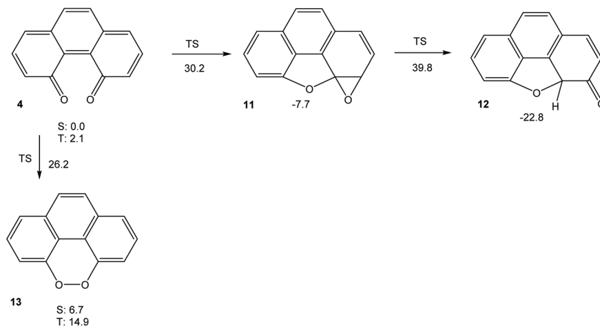
Fig. 3 Free energies (in kcal mol -1 ) of relevant stationary points on the potential energy hypersurface of 4 (M06-2X/cc-pVTZ). All stationary points are on the singlet spin manifold, unless indicated otherwise.
