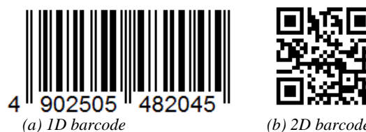
Figure 1: Example of 1D and 2D barcodes
