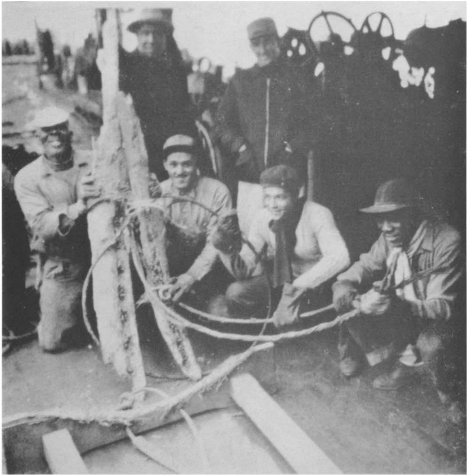
Fig. 6. Photograph of whale's jaw and mauled cable brought up from 620 fathoms off Peru on October 14th, 1955. (See Appendix, No. 14).
