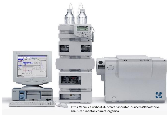
Figure 17. Configuration of an Agilent LC/MSD VL mass spectrometer coupled to the HPLC device
