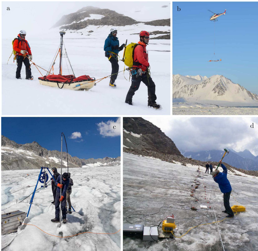
Figure 1. Field photographs illustrating different methods for measuring glacier thickness. (a) Ground-penetrating radar measurements on Johnsons Glacier, Antarctica, in January 2020. The white sledge contains a radar transmitter, receiver, shielded antennas, control unit, and recording system. A Global Navigation Satellite System receiver antenna is mounted to the sledge. Credit: Francisco Navarro. (b) Aerial ground-penetrating radar measurements over Hansbreen, Svalbard, in spring 2011 (Navarro et al., 2014). The radar transmitter, receiver, and antennas are mounted to a wooden frame hung from the helicopter. Credit: Antoine Kies. (c) Hot water drilling on Rhonegletscher, Switzerland, in August 2018 by ETH Zurich’s Glacier Seismology Group. Although used mostly for characterizing bed conditions, the drillings measure ice thickness as a side product. Credit: Johannes Landmann. (d) Seismic reflection measurements on Grubengletscher, Switzerland, using a sledgemoor as a seismic energy source. The black seismic line connects geophones to the recording system. Credit: Bernd Kulesa.
