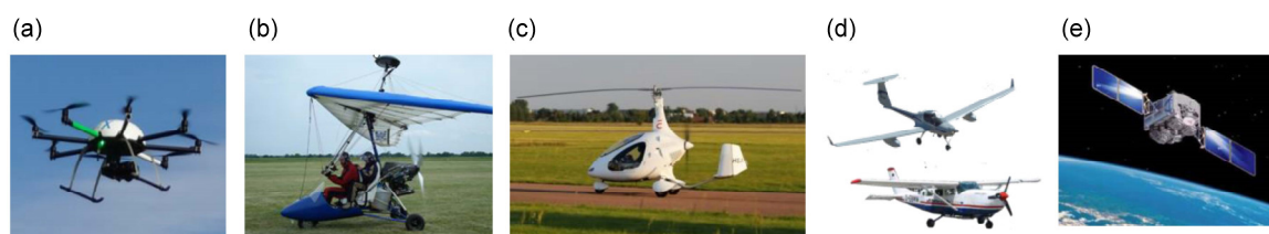
Figure 1. Different air- and spaceborne remote sensing platforms for assessing geomorphological landforms and their traits: (a) unmanned aerial vehicles (UAVs) or drones, (b) microlight-gravity-controlled aircrafts (c) gyrocopter-microlight helicopter, (d) ECO-Dimona aircraft (top) and Cessna aircraft (bottom), and (e) satellite (from Lausch et al. [3]).
