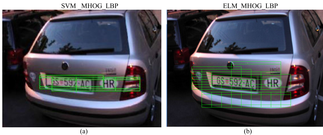
FIGURE 11. (a) The output of the proposed method using the SVM without the mean-shift algorithm; (b) The output of the proposed method using the ELM without the mean-shift algorithm.
