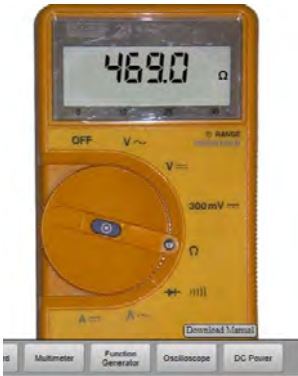
Figure 4 - Multimeter Detail (VISIR System)
