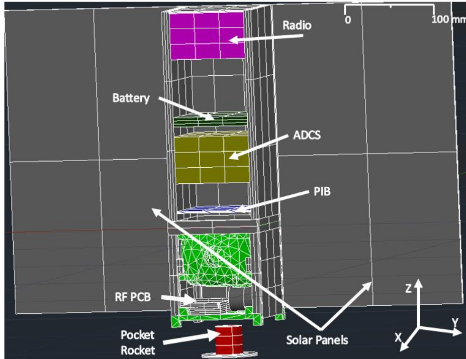
Figure 4.22: 2U Interfacing CubeSat generic geometry with Propulsion Module and Side Paneling removed
