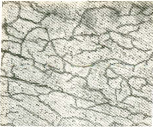
Fig. 1(g): Structure of chromium deposited on Bright nickel ( \times 1000 )
