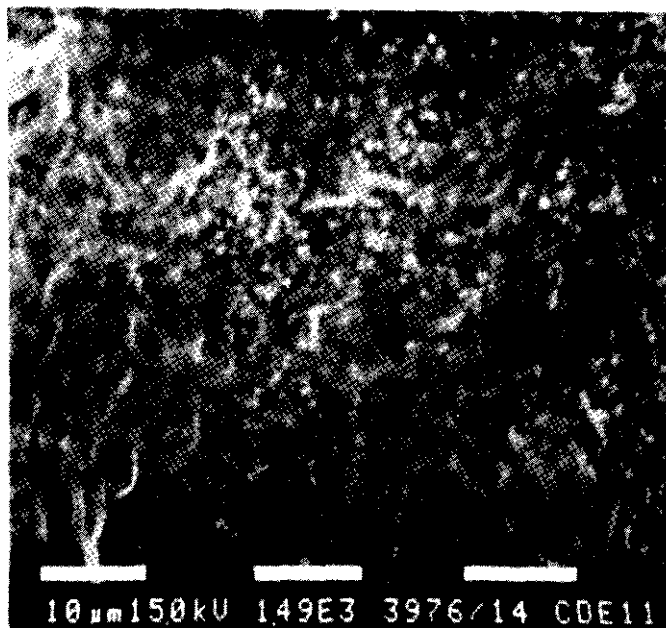
Fig. 3 (b): Scanning electron micrographs of \text{Cu}_{1.72}\text{Se} layer after heat treatment X 1490
