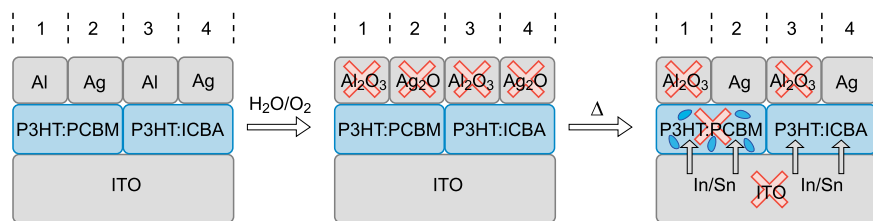
FIG. 6. A schematic of device degradation pathways (indicated by the red crosses) in devices with (1) Al cathode, P3HT:PCBM active layer and ITO anode; (2) Ag cathode, P3HT:PCBM active layer and ITO anode; (3) Al cathode, P3HT:ICBA active layer and ITO anode; and (4) Ag cathode, P3HT:ICBA active layer and ITO anode, upon exposure to water and oxygen and subsequent thermal regeneration.
