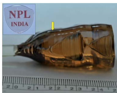
Fig. 2 Fe-doped \text{LiNbO}_3 single crystal grown along [001] . Inset shows a Z-cut and optically polished wafer from the region of boule indicated by the arrow.
