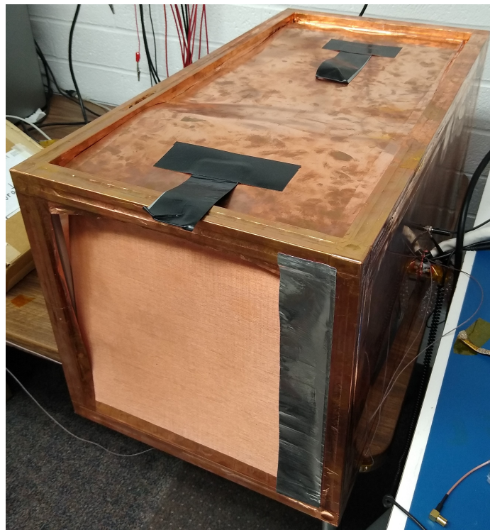
Fig. 3.3: Faraday Cage used to Test GRIDS
