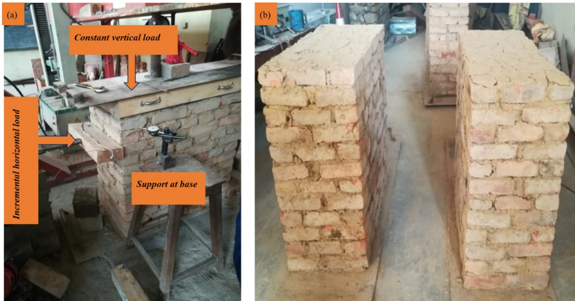
137 Fig. 2 a) Experimental setup for in-plane shear test showing loading direction, b) wall 138 samples prepared for in-plane shear test
