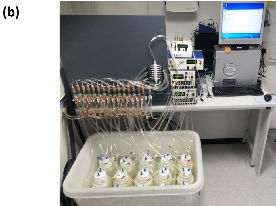
Figure 5.2.1 Experimental set-up for biodegradation test. (a) Schematic diagram of respirometric system components; (b) The original laboratory set-up of the respirometric system
