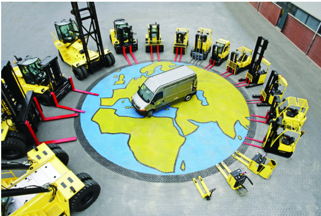
Figure 1.1: Materials handling trucks from smallest (hand pallet truck) to largest (reachstacker)
