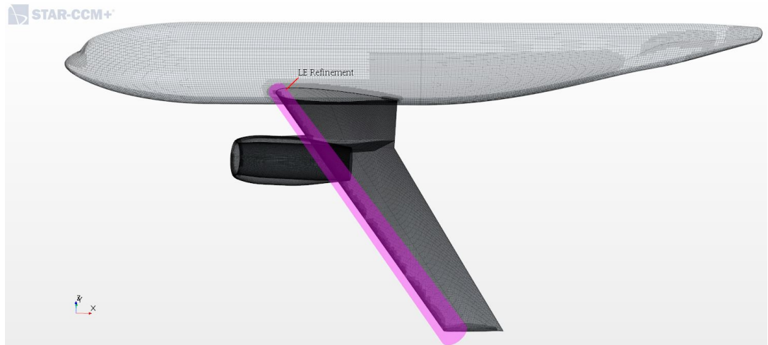
Figure 4.3: Illustration of an example of cylinder-shaped mesh refinement zone (purple) across the leading edge.
