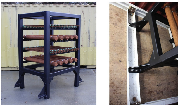
Fig. 7. Pipe rack (left) and brackets fixed to frame inside the container (right).
