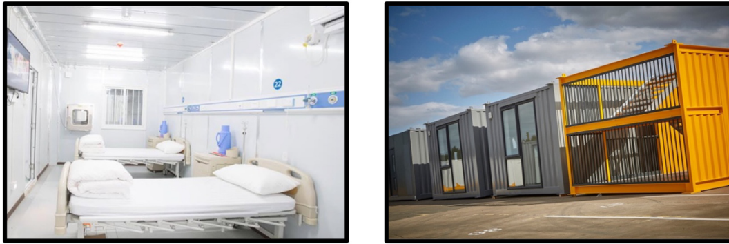
Fig. 7. Examples of emergency modular isolation units.
