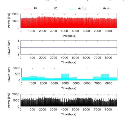
Fig. 14. Energy contribution for the HRES components (NRU<sup>max</sup> =100%, scenario 1).
