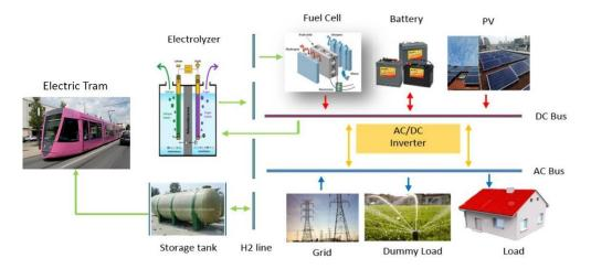
Fig. 3. Schematic of the studied grid-connected PV/H<sub>2</sub> hybrid system.
