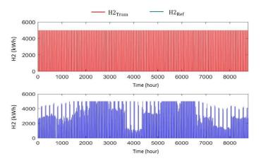
Fig. 19. The refuelled H<sub>2</sub> by the system and the H<sub>2</sub> required by the tram (in case of integrating three trams).
