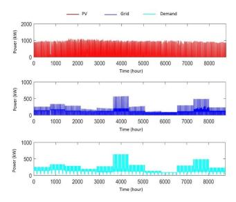
Fig. 18. The contribution of the PV system and the grid (in case of integrating three trams).
