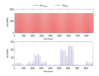
Fig. 17. The refuelled H<sub>2</sub> by the system and the H<sub>2</sub> required by the tram (in case of integrating one tram).
