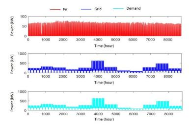
Fig. 16. The contribution of the PV system and the grid (in case of integrating one tram).
