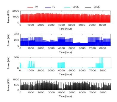
Fig. 15. Energy contribution to the HRES's components (NRU<sup>max</sup> =1%, Scenario 1).
