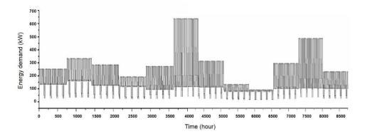
Fig. 5. Campus building's yearly load profile (considering five working days in a week).
