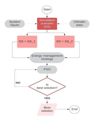
Fig. 9. The block diagram for the proposed optimization framework with two simulation scenarios.
