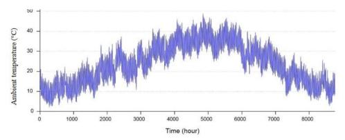
Fig. 7. Hourly ambient temperature at the building location over one year (Ouargla, Algeria).
