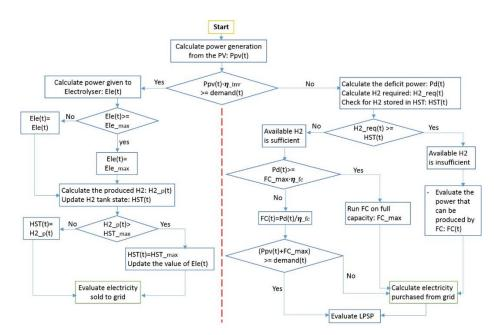
Fig. 10. Schematic of the studied grid-connected PV-H<sub>2</sub> hybrid system without sector coupling strategy (Scenario 1).
