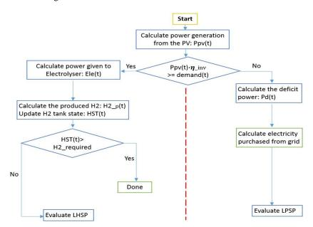
Fig. 12. Flow chart for the energy management using sector coupling strategy (Scenario 2).
