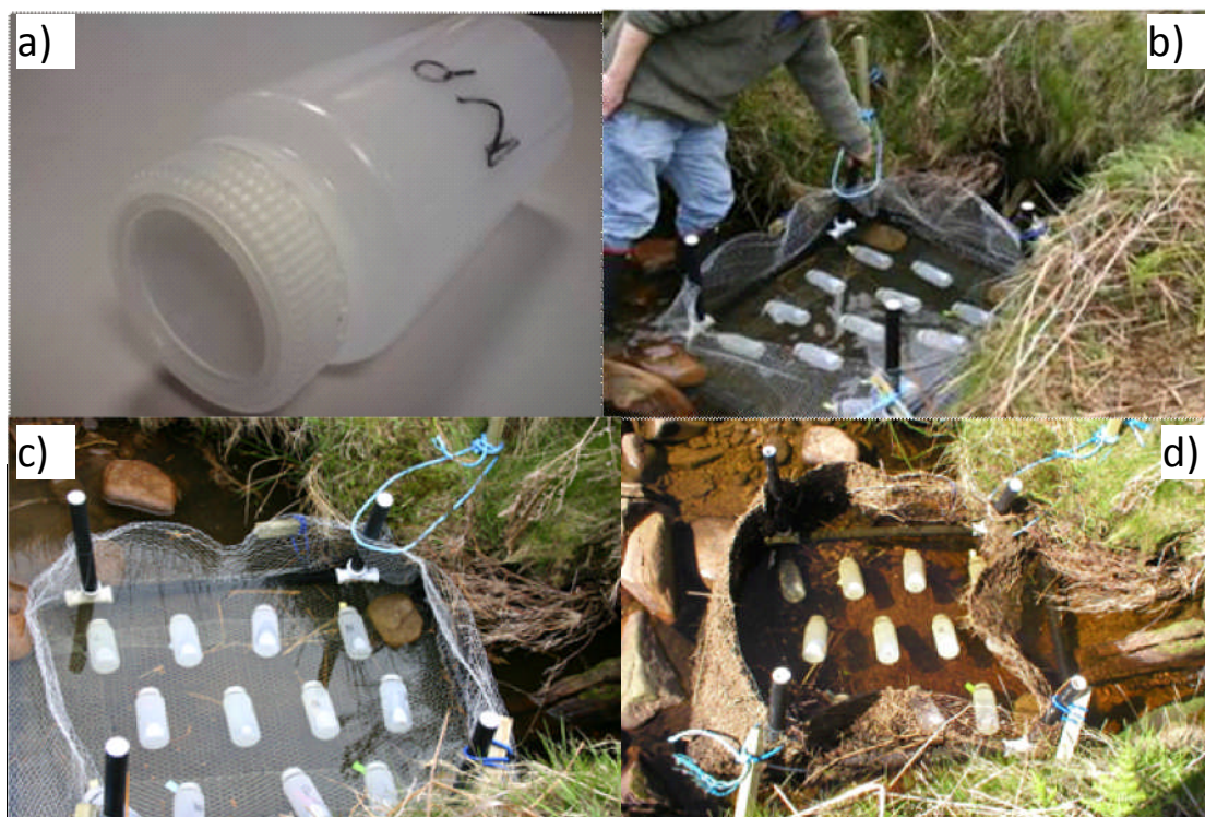
Figure 2.2.1: The periphytometer in the laboratory and at the River Etherow: a) single bottle showing cut-lid replaced with glass-fibre filter; b) installing the frame in the Etherow; c) the installed frame, note filters are orientated parallel to the flow; d) the frame at the end of the incubation.
