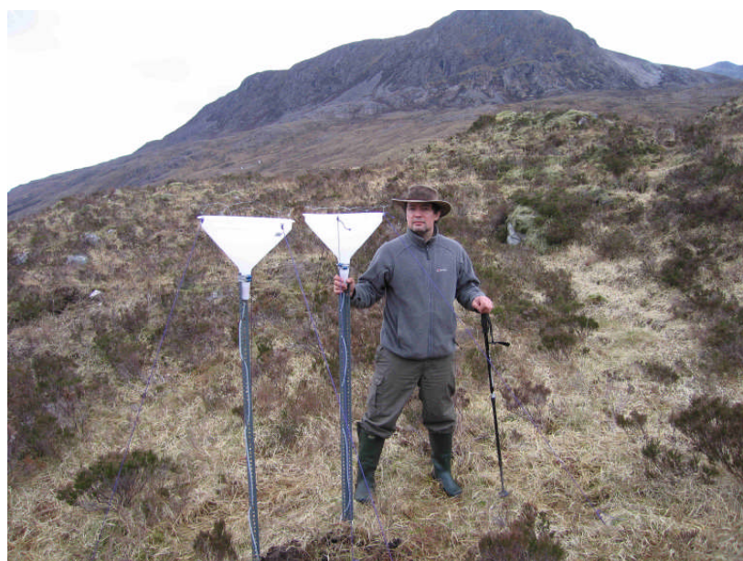
Figure 4.1.2: High volume bulk deposition samplers for \text{NH}_4^+ and \text{NO}_3^- , Loch Coire Fionnaraich
