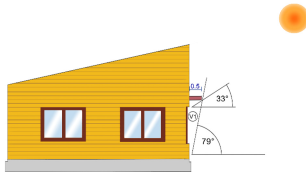
Figure 6. Shading produced by eaves on the north façade of the building. Own elaboration.
