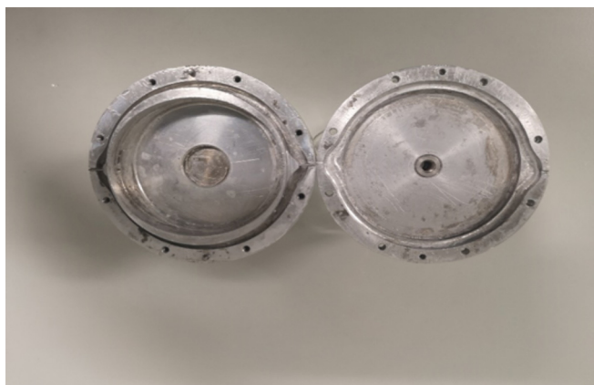
FIG. 14. Two halves of the novel setup making the co-axial pressurized gyration device. Reproduced with permission from S. Mahalingam, S. Homer-Vanniasinkam, and M. Edirisinghe, “Novel pressurized gyration device for making core–sheath polymer fibers,” Mater. Des. 178 , 107846 (2019). Copyright 2019 licensed under a Creative Commons Attribution (CC BY) license.
