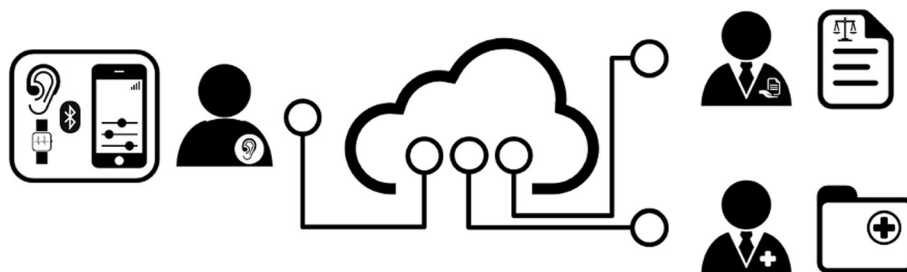
Fig. 1 Schematic representation of the EVOTION platform. Middle: the EVOTION Data Repository collecting data from various sources. Left: Hearing aid users transmitting data via smart hearing aids, smartphones and potentially via smartwatches if available using a Bluetooth connection. Bottom right: healthcare professional entering data from the clinic either directly through a dashboard of the platform or through existing clinical databases connected to the EVOTION Data Repository. Top right: policy-maker running queries on the EVOTION database through the dashboard in order to answer specific public health issues. Source: Pontoppidan 2019 [27]. Used with permission
