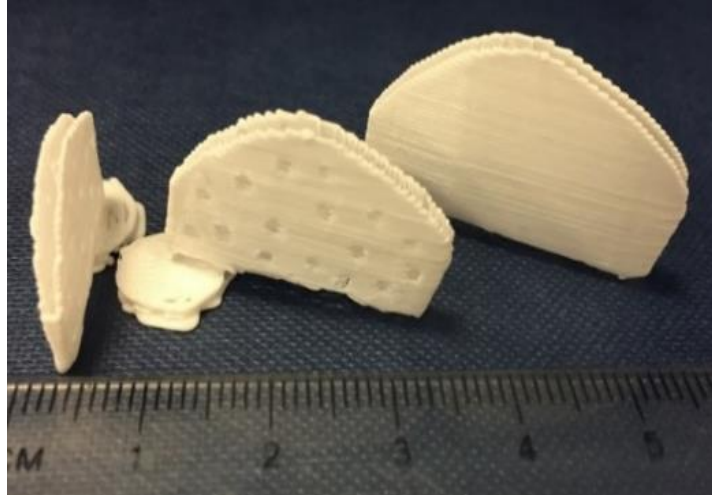
Figure 4.22. Photograph of PLA septal pockets printed with PLA filament to full scale. Pockets with and without holes were printed with good fidelity.
