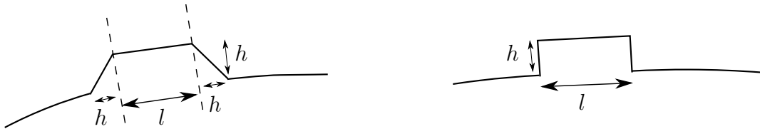
Figure 6.1: Schematic showing ramped edge bump compared to the vertical edge bump case, where l denotes the length of the bump and h the height.
