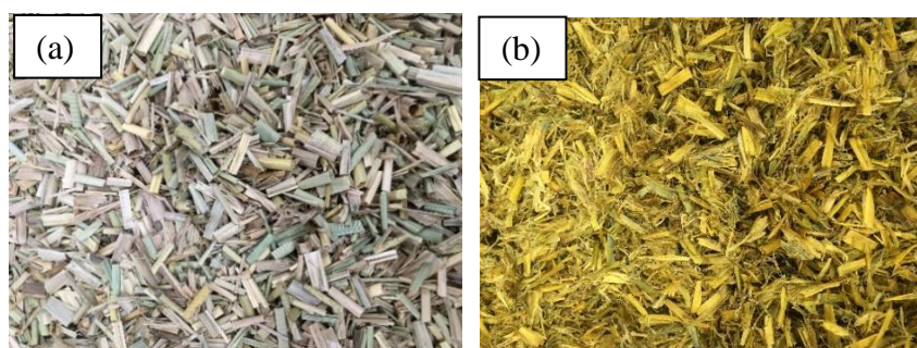
Fig. 2. (a) Untreated and (b) treated rice straw fibres
