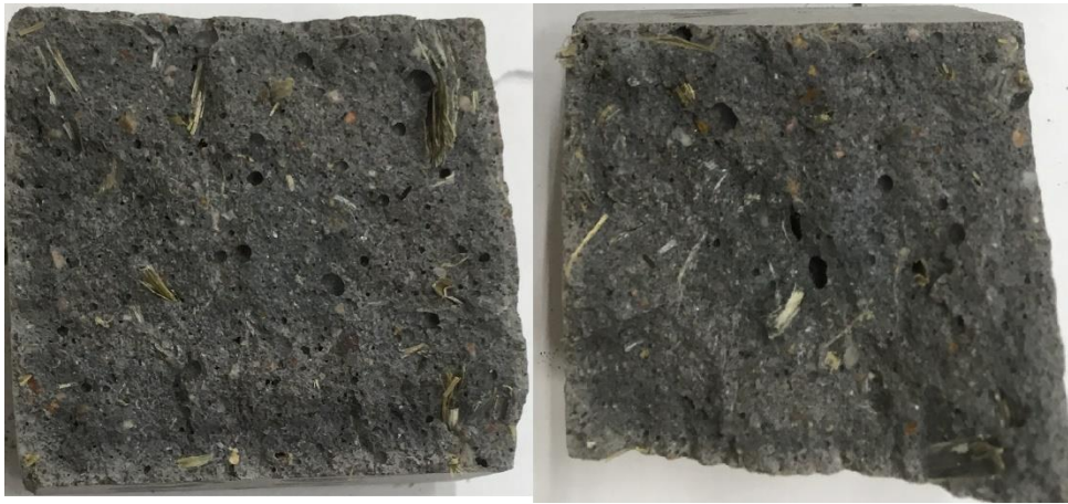
500 Fig. 16. Failures of treated rice straw after 20 wet/dry cycles under flexural testing
