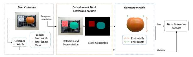
**Figure 1.** (Best viewed in color). Step-by-step illustration of our detection and instance-based segmentation system with dimension and mass estimation of tomato fruits.
