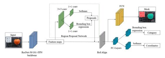
**Figure 3.** Complete Mask-RCNN framework with three stages: a feature extraction backbone network, a region proposal network (RPN) to generate RoIs (region of interests), and an FCN (fully convoluted network) running parallel to fully connected networks to extract instance-wise semantic masks and to perform target detection with classification outputs.
