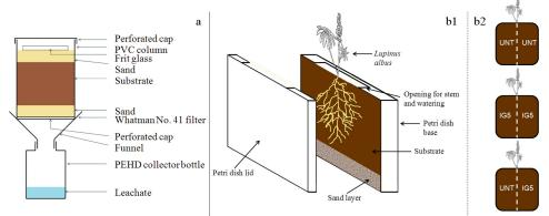
Figure 1. Design of the leaching column (a) and rhizobox (b1) and experimental designs (b2).
