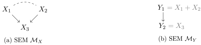
Figure 5.2 Graphical illustration of parent-child relationships for the examples in Section 5.5.5. The micro-level model \mathcal{M}_X depicted in (a) is to be transformed into the macro-level model \mathcal{M}_Y depicted in (b) which is a coarser descriptions as in it only considers the sum of X_1 and X_2 . In Section 5.5.5 we give examples of what can go wrong if the transformation is not exact.
