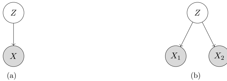
Figure 4.1 Graphical models depicting (a) the usual single-view ICA setting; (2) the multi-view setting considered in this work. Z is a vector of unobserved latent sources and the X_i are observed mixtures of the components of Z . In both settings, all variables are of the same dimension.
