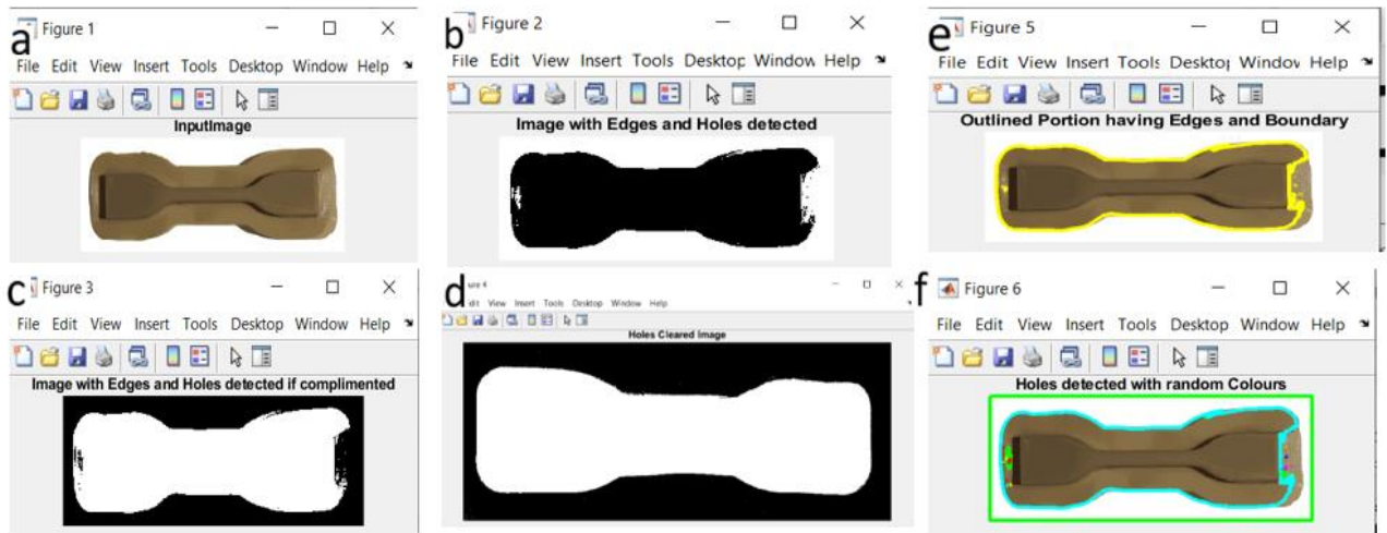
Fig.6 Processing steps of Pores detection for an image without defect (a) Input image; (b) Complemented image of a sample; (c) Binary image of sample exposing every defect (d) Complemented Images of Samples with all holes/defect filled. (e) Outline of the boundaries of samples traced by code (f) Result of local pores detection
