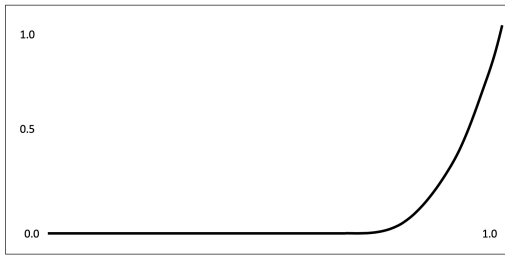
Figure 9: Animation Curve used to dictate how each part of the endoscope moves, allowing the most movement at the tip of the endoscope. X-Axis (0.0 to 1.0) is position on the endoscope, Y-Axis (0.0 to 1.0) is amount of movement
