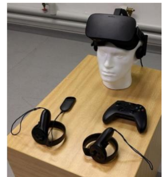
Figure 2. The Oculus Rift HMD with its interaction devices including wireless hand controllers
