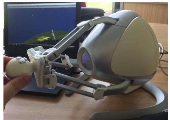
Figure 3: The Novint Falcon being used to control a virtual needle in ParaVR
