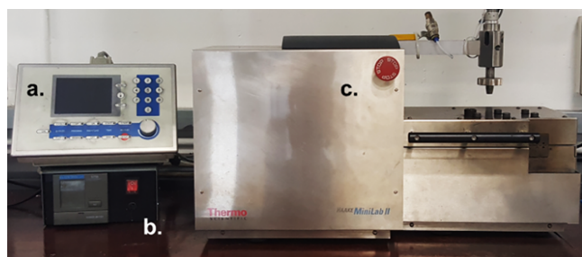
FIGURE 6 Twin-screw extruder with other experimental equipment. A, Power meter, B, Interface control system, and C, Haake MiniLab [Color figure can be viewed at wileyonlinelibrary.com]
