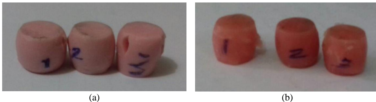
Figure 11. Failed specimens made of acrylic resins with TiO 2 nanoparticles: (a) cold cure and (b) heat cure.
