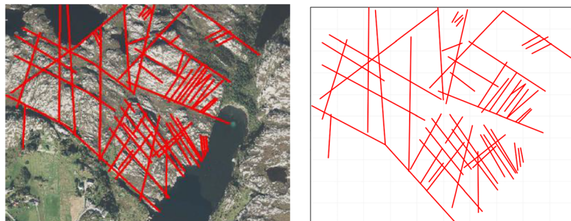
Figure 11. Fracture set in a confined aquifer modified from the work of Flemisch et al. (2017).
