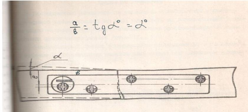
Figure 11. Diagram of calculation of deflection angle
