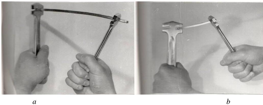
*Figure 4. Variants (a, b) of modeling bone fixing device depending on the shape of the segment.*
