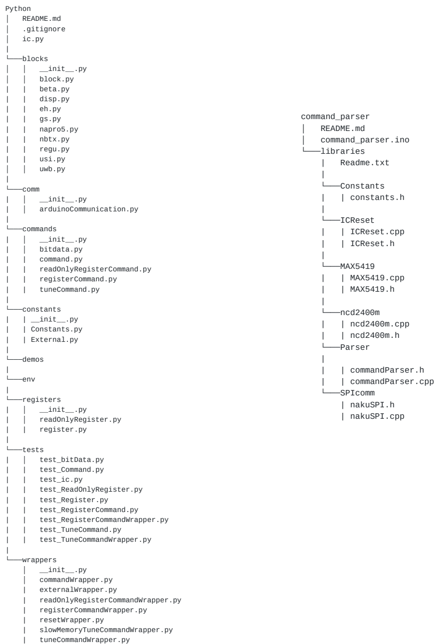
Figure 52: IC Communication software structure.
