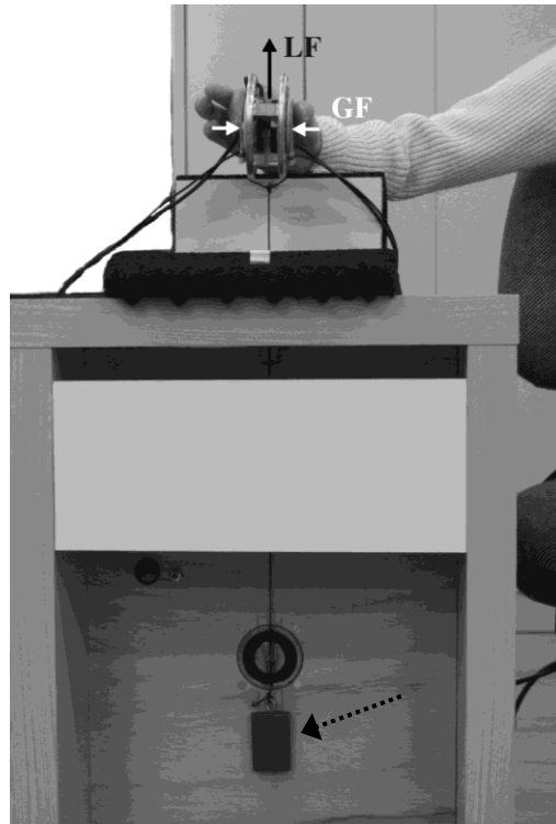
Figure II.1. Handheld object used to measure the different forces during the task. Grip force (GF) normal to the contact surfaces is indicated by white arrows, tangential load force (LF) by a black arrow and the steel mass by a dotted arrow.
