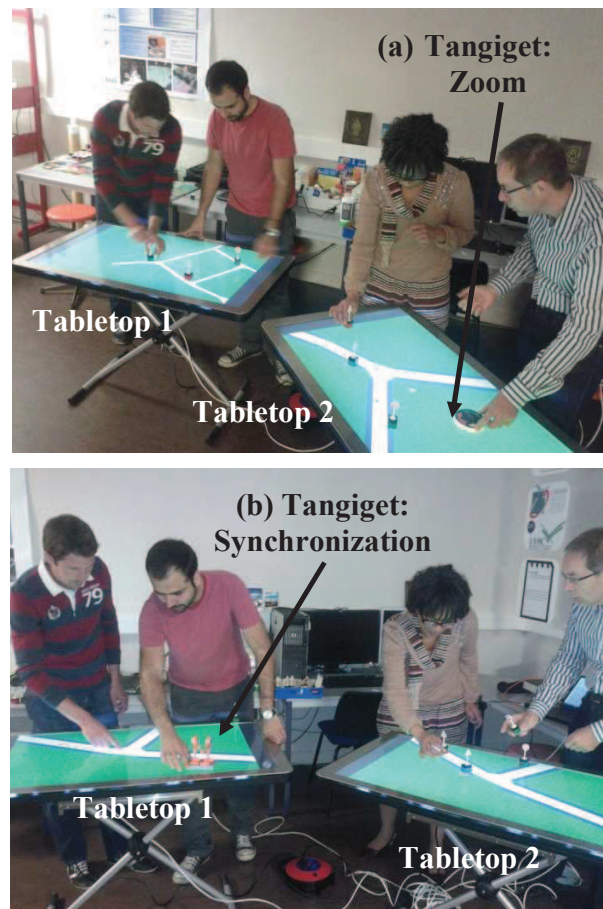
Figure 2. Road traffic management on two TangiSense with Tangigets (a) without effect on the other tabletop, (b) with effect on it
